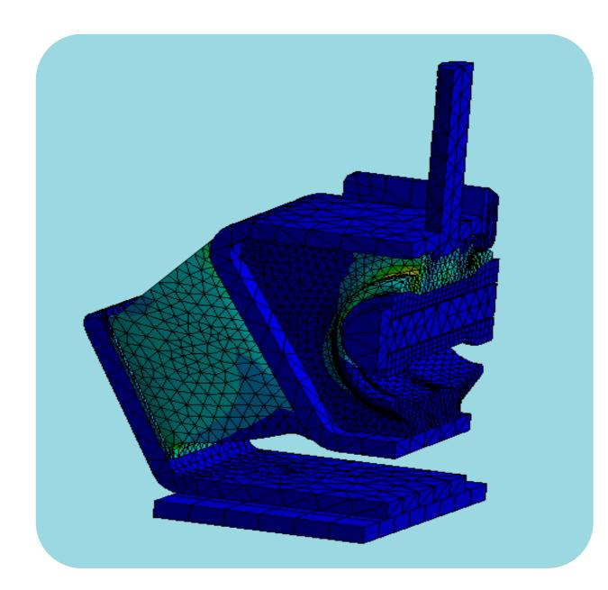
The non-linear characteristics of the material used cannot be approximated due the large deformations
